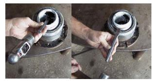
Split the inside of bushing with a chisel. Tap bushing up and out. Gently chisel around top of bearing to remove hardened concrete. Lubricate bearing to free up.
