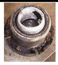
Remove excess build up from inside (below left). Tapered Line up nose (top center below) may be found in bottom. It is no longer needed and may be discarded.
